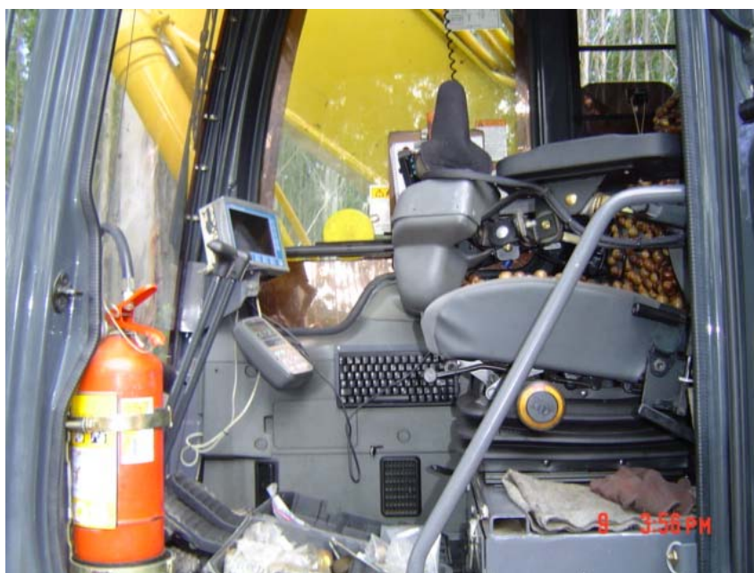
Fig 3.4 – Cabine de controle do processador Harvester Komatsu 02
