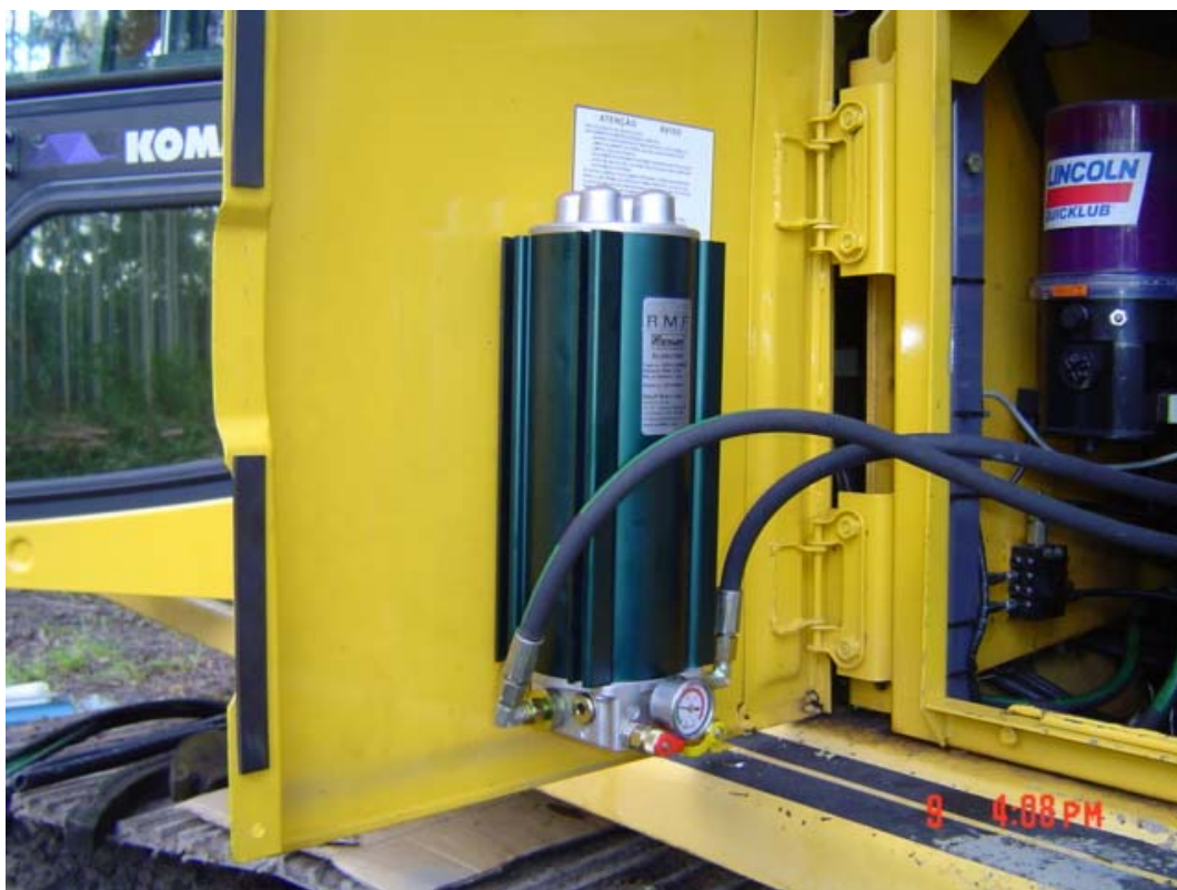
Fig 3.2 – Filtro By-Pass RMF Komatsu 02
