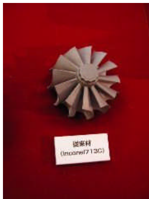
FIGURA 20 – Turbo Compressor de Inconel 713C, Ni-2Nb-12.5%Cr-4.2%Mo-0.8%Ti-6.1%Al-0.12%C-0.012%B-0.1%Zr [24].
